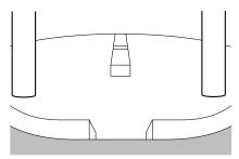
The area above the camera cannot be viewed. If there is an object that has a wide projection on its upper part such as a sign pole behind the vehicle, the projection cannot be seen on the screen.
