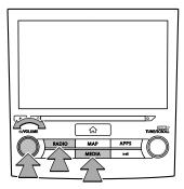
"O/VOLUME" knob: Press and hold to turn the audio system off, and press to turn it on again. The system turns on in the last mode used. Turn this knob to adjust the volume. Press to mute the audio system.
