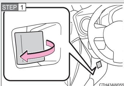
Pull the engine hood release lever.
