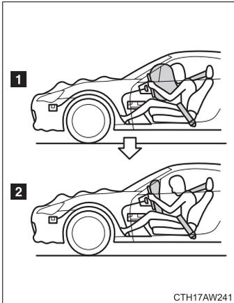
**1** SRS AIRBAGs deploy as soon as a collision occurs.
