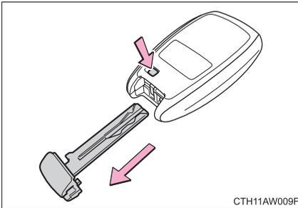
To take out the mechanical key, push the release knob and take the key out.
