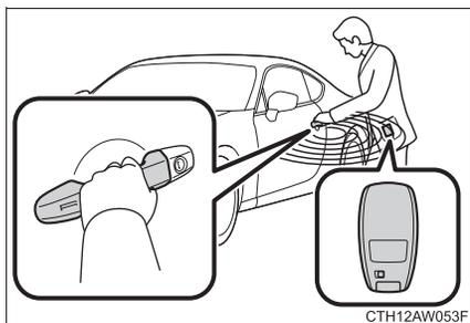
Grip the driver's door handle to unlock the door. Grip the passenger's door handle to unlock all the doors.
