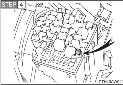
Remove the fuse with the pull-out tool.
