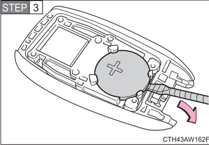
Remove the depleted battery.
