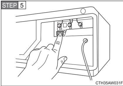
At the garage door opener motor, (security gate motor, etc...) locate the “Learn”, “Smart”, or “Program” button. This can usually be found where the hanging antenna wire is attached to the motor-head unit (see the device’s manual to identify this button). The name and color of the button may vary by manufacturer.
