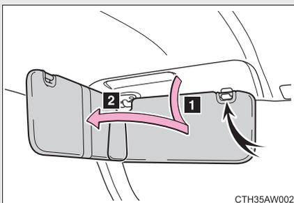
**1** To set the visor in the forward position, flip it down.
