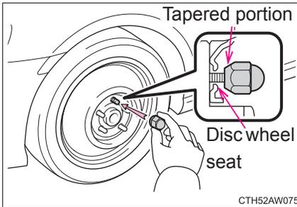
Vehicles with a compact spare tire: Tighten the wheel nuts until the tapered portion comes into loose contact with the disc wheel seat.
