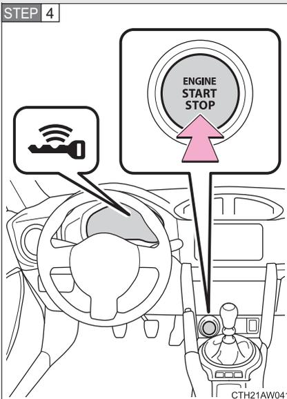
Press the push-button ignition switch shortly and firmly.
