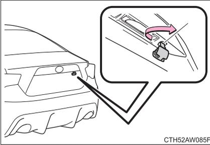
Turn the mechanical key clockwise to open.
