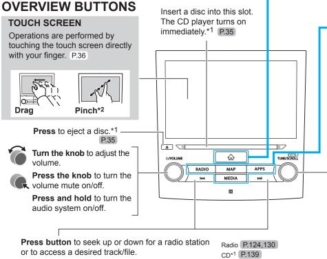
Press and hold button to continuously seek for a radio station, or to fast forward/rewind files or tracks. B
