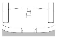
The area above the camera cannot be viewed. If there is an object that has a wide projection on its upper part such as a sign pole behind the vehicle, the projection cannot be seen on the screen.
