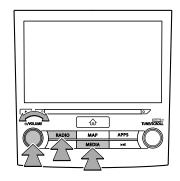
"<sup>(h</sup>/VOLUME" knob: Press and hold to turn the audio system on and off. The system turns on in the last mode used. Turn this knob to adjust the volume.
