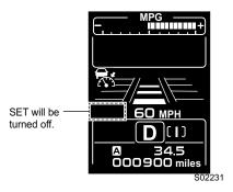
• Press the 🗟 (CRUISE) switch. SET will be turned off while the set vehicle target speed remains displayed on the EyeSight display area.
