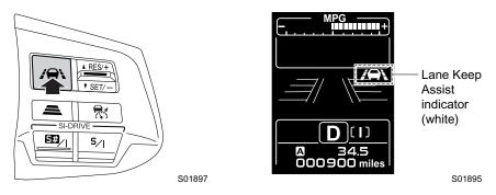
Press the Asist (Lane Keep Assist) switch once again to turn it off, and " T (Lane Keep Assist indicator) is turned off on the EyeSight display area.
