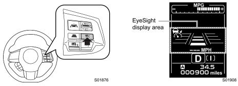
If the switch is pressed once more, the EyeSight display will turn off. It will also automatically turn off when the engine is stopped.
