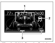
When the Vehicle Dynamics Control system activates, the tires illuminate in yellow and the Vehicle Dynamics Control system operating indicator flashes.
