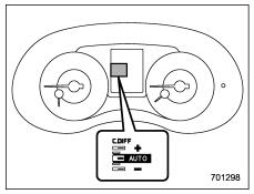
This indicator functions while the ignition switch is "ON". When it appears, it indicates that the driver's control center differential is set to the auto mode. It disappears when the driver's control center differential is set to the manual
