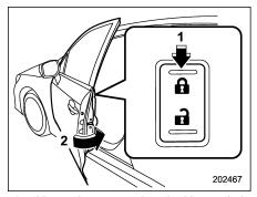
Locking using power door locking switch
