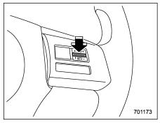
Press the "RES/SET" switch to the "SFT" side and hold it until the vehicle reaches the desired speed. Then, release the switch. The vehicle speed at that moment will be memorized and treated as the new set speed.
