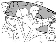
The SRS side airbag is stored in the door side of each front seat seatback.
