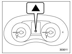
When the Intelligent (I) mode is selected, a shift-up indicator "A" on the combination meter will blink to signal the best time to shift gears for maximum fuel efficiency.
