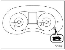
When the Hill Holder function is activated. the Hill Holder indicator light illuminates. Refer to "Hill Holder indicator light (models with electronic parking brake system)" **3-24**
