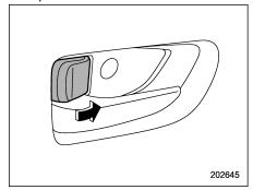
Rotate the lock lever forward.
