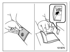
Remove the covers and locate the lower anchorages (bars).
