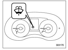
When there is only a small amount of washer fluid remaining, the windshield washer fluid warning indicator will illuminate. When this occurs, refill the washer fluid as follows.
