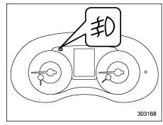
The indicator light on the combination meter will illuminate when the front foa lights are illuminated.
