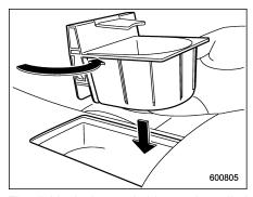
The divider in the cup holder can be pulled out and inserted in a different position (further toward the front or rear) to enable cups of different sizes to be held.
