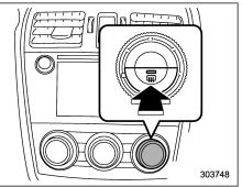
To activate the defogger and deicer system, press the control switch that is located on the climate control panel. The rear window defogger, outside mirror defogger and windshield wiper deicer are activated simultaneously. The indicator light on the control switch illuminates while the defogger and deicer system is activated.
