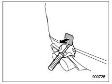
2. Pry off the cover on the rear bumper using a screwdriver, and you will find a
