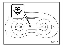
The windshield washer fluid warning indicator appears when the washer fluid level in the tank has dropped to the lower limit. If the warning indicator appears, refill the tank with fluid. For the refilling procedure, refer to "Windshield washer fluid" @ 11-38.
