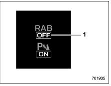
Reverse Automatic Braking system OFF indicator
