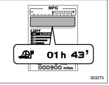
This screen displays the journey time (the time that has elapsed since the ignition switch was turned to the "ON" position).
