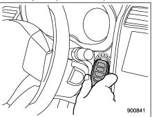
4. Hold the access key with the buttons facing you, and touch the push-button ignition switch with it.
