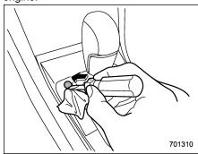
2. Wrap the tip of a flat-head screwdriver with vinvl tape or a cloth and use it to remove the shift lock cover. The shift lock release button is located under the shift lock cover.
