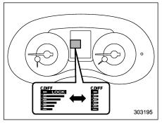
All the indicators will flash in the event that the driver's control center differential has a malfunction. Have the vehicle inspected by your SUBARU dealer. For details, refer to "Driver's Control Center Differential (C. DIFF/DCCD) (STI)" @7-19.
