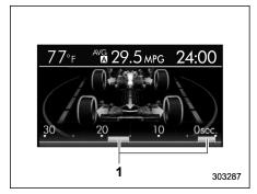
When the Vehicle Dynamics Control system starts to activate, the tires illuminate in yellow.
