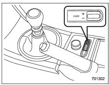
The control switch is located beside the parking brake lever. By pushing the control switch forward or pulling it rearward, it is possible to change the initial LSD torque.
