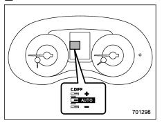
In the auto mode, the system estimates the driving and road conditions using signals from the wheel speed sensor, throttle position sensor, steering angle sensor and brake switch, etc. According to the result, it electronically and automatically controls the degree of limitation of the differential action (LSD torque) to optimize the differential action of the center differential. When the ignition switch is turned ON, the "AUTO" indicator on the combination meter appears.
