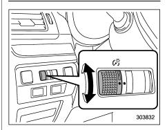
You can adjust the illumination brightness of the combination meter, the climate control panel, etc. by turning the control dial.
