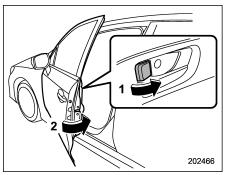
Locking using lock lever
