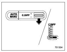
Pull the switch rearward to reduce the initial LSD torque. When the lowest position of the driver's control center differential indicator is displayed, the initial LSD torque will be minimum. Under this condition, only the Mechanical LSD torque will limit the differential action.
