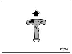
To open the trunk lid from inside the trunk. pull the yellow handle as indicated by the arrow on the handle. This operation unlocks the trunk lid. Then, push up the
