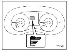
When you select the manual mode of the driver's control center differential, the initial limited slip differential (LSD) torque that is currently selected for the center differential is indicated by the illumination of these indicator.
