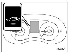
When the door is unlocked, and the driver's door is opened and then closed, the welcome screen will appear for approximately 20 seconds.
