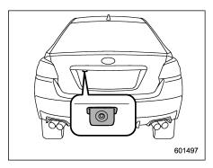
A rear view camera is attached to the trunk lid. When the ignition switch is "ON" and the shift lever (MT models) or select lever (CVT models) is set to "R", the rear view camera automatically displays the rear view image behind the vehicle on the monitor of the navigation system or the audio display.
