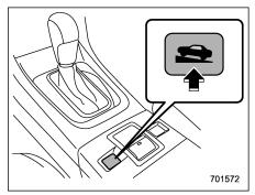
You can activate/deactivate the Hill Holder function by pressing the Hill Holder switch.
