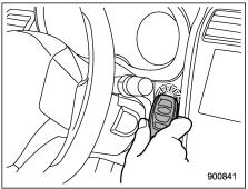
5. Hold the access key with the buttons facing you, and touch the push-button ignition switch with it.
