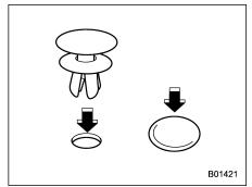
Insert the clip without the head first and then push the head of the clip into the hole.
