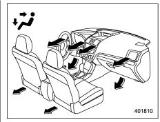
(Bi-level): Instrument panel outlets and foot outlets
