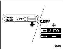
Pull the control switch rearward to select the "AUTO [-]" mode. After setting the mode, "AUTO [-]" appears.
