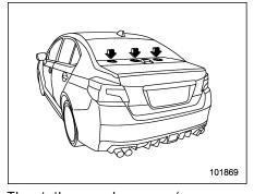
The tether anchorages (upper anchorages) are provided at the locations shown in the above illustration. For details, refer to "Top tether anchorages" @ 1-32.
