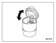
The portable ashtray can be installed in each cup holder or bottle holder. For the locations of the cup holders, refer to "Cup holders" \$\alpha\$6-6. For the locations of the bottle holders, refer to "Bottle holders" @6-7.
