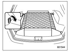
The cargo area is equipped with four tiedown hooks so that cargo can be secured with a luggage net or ropes.
