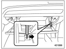
(2) Remove the damper shaft from the glove box.
