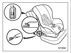
Some types of child restraint systems can be installed on the rear seat of your vehicle without use of the seatbelts. Such child restraint systems are secured to the dedicated anchorages provided on the vehicle body.
