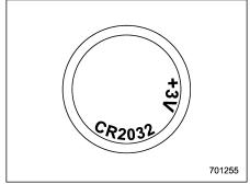
3. Remove the circuit board from the bottom half of the case and remove the battery and replace with a new one. Be sure to observe the (+) sign on the old battery before removing it to ensure that the new battery is inserted properly
