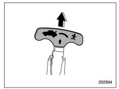
To open the trunk lid from inside the trunk, pull the yellow handle as indicated by the arrow on the handle. This operation unlocks the trunk lid. Then, push up the lid.
