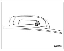
The coat hook is attached to each rear passenger's hand grip.
