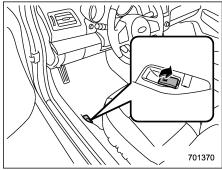
2. To open the fuel filler lid, pull the lid release lever up. The lever is on the floor at the left of the driver's seat.
