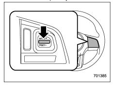
2. When the speed decreases to the desired speed, press the "RES/SET" switch to the "SET" side once. Now the desired speed is set and the vehicle will keep running at that speed without depressing the accelerator pedal.
