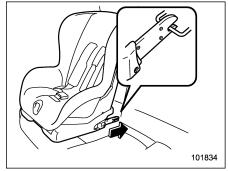
1. While following the instructions supplied by the child restraint system manufacturer, connect the lower hooks onto the lower anchorages located at "©" marks on the bottom of the rear seatback. When the hooks are connected, make sure the adjacent seatbelts are not caught.
