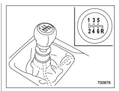
The manual transmission is a full synchromesh, 6-forward-speed and 1-reversespeed transmission.
