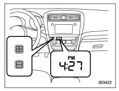
The clock shows the time while the ignition switch is in the "ACC" or "ON" position.
