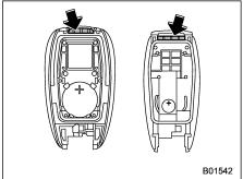
5. Attach the cover to the access key by fitting the projections and recesses together.
