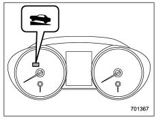
When the Hill Holder function is activated, the Hill Holder indicator light illuminates. Refer to "Hill Holder indicator light" \$\tilde{\sigma}\$-21.
