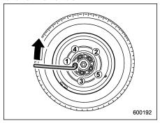
16. Use the wheel nut wrench to securely tighten the wheel nuts to the specified torque, following the tightening order in the illustration.
