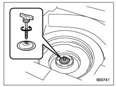
6. Take out the under-floor storage compartment and turn the attaching bolt counterclockwise, then take the spare tire out.
