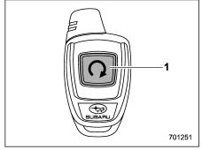
Remote engine starter transceiver (fob)
