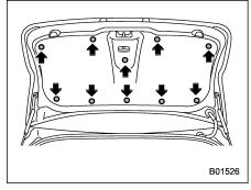
2. Remove the trunk trim lining by removing the clips indicated in the illustration.
