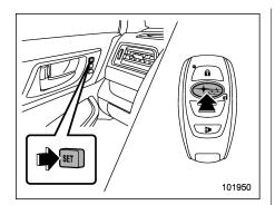
2. While holding the access key and pressing the "SET" button, press the "♣" button of the access key.
