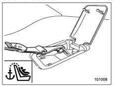
4. Fasten the top tether hook of the child restraint system to the appropriate upper
