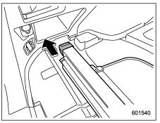
5. Insert the left end of the cover housing into the retainer.
