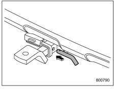
2. Insert the hitch pin into the hole located on the hitch receiver tube so that the pin passes through the ball mount.
