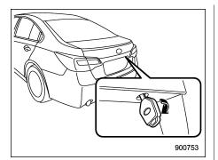
To open the trunk lid, insert the key into the key cylinder and turn it clockwise.
