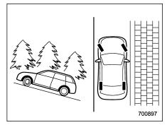
When parking on a hill, always turn the steering wheel as described here. When the vehicle is headed up the hill, the front wheels should be turned away from the curb.
