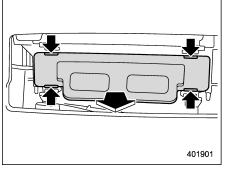
2. Remove the cover of the air filter.
