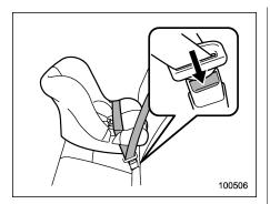
8. To remove the child restraint system, press the release button on the seatbelt buckle and allow the belt to retract completely. The belt will return to the FIR mode.
