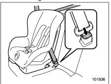
12. To remove the child restraint system, press the release button on the seatbelt buckle and allow the belt to retract completely. The belt will return to the FLR mode
