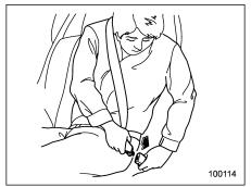
5. Insert the center seatbelt tongue plate into the center seatbelt buckle until it
