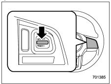
2. Press the "RES/SET" switch to the "SET" side once. Now the desired speed
