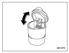
The portable ashtray can be installed in each cup holder. For the locations of the cup holders, refer to "Cup holder" \$\alpha\$6-8. When using the ashtray, open the lid of the ashtray. When removing the ashtray from a cup holder, pull the ashtray upwards. Fully close the lid after using the ashtray to help reduce residual smoke.
