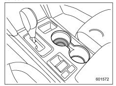
The bottle stopper is equipped to stabilize a small cup, bottle or can. Remove it if it is not being used.
