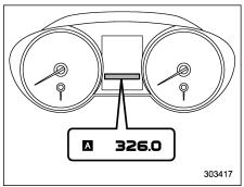
This meter displays the two trip meters when the ignition switch is in the "ON" position.
