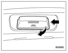
1. To remove the right-hand side license plate light cover, insert a finger into the right side of the cover, and then press once to the left and pull it out. To remove the left-hand side license plate light cover, insert a finger into the left side of the cover, and then press once to the right and pull it out.
