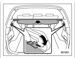
2. Pull the handle toward you to extend the cargo area cover. Then insert its hooks into the catches as shown.
