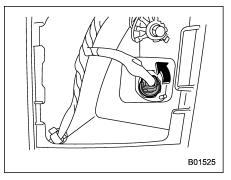
2. Turn the bulb socket counterclockwise and remove it.
