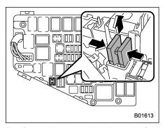
The fuse puller is stored in the main fuse box in the engine compartment. To pick up the fuse puller, pull it out while pinching the puller head with your fingers.
