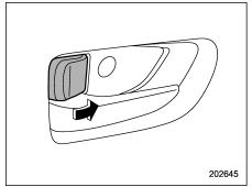
2. Rotate the lock lever forward.
