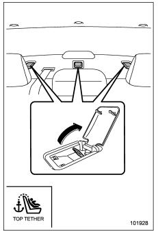
Three tether anchorages are installed on the rear shelf behind the rear seat head restraint. Open the cover flap to use each anchorage.
