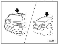
The satellite antenna and STARLINK antenna (if equipped) are installed in the center of the roof at the rear.
