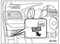
2. Pull the hood lock release knob under the instrument panel.
