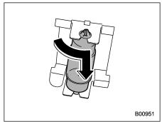
2. Turn the bulb until the flat surfaces at its ends are aligned vertically.
