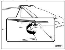
3. Remove the bolt of the crossbar by using the torque wrench.
