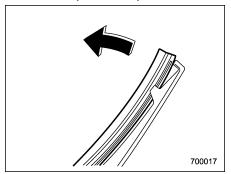
1. Pull out the end of the blade rubber assembly to unlock it from the plastic support.
