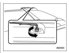
2. Remove the cap of the roof rail holder by using the torque wrench.
