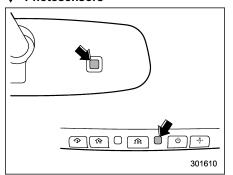
The mirror has a photosensor attached on both the front and back sides. During nighttime driving, these sensors detect distracting glare from vehicle headlights behind you and automatically dim the mirror to eliminate glare and preserve vour vision. For this reason, use care not to cover the sensors with stickers, or other similar items. Periodically wipe the sensors clean using a piece of dry soft cotton cloth or an applicator.
