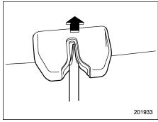
2. Use a flat-head screwdriver with a thin blade. Slide the flat-head screwdriver blade from the slit aperture of the lock assembly fully to the end until you hear a click.
