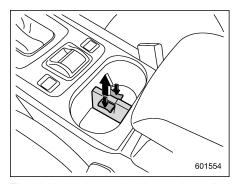
The divider in the cup holder can be pulled out. With the divider taken out, the cup holder can be used as a storage box.
