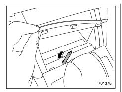
5. While depressing the brake pedal, insert the screwdriver into the hole, press the shift lock release portion using the screwdriver, and then move the select lever.
