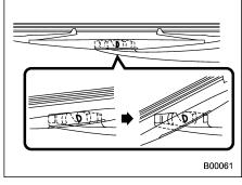
2. Turn the wiper blade assembly counterclockwise.
