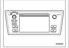
Press the power/VOLUME knob to turn the audio/visual system on and off. When the system turns on, the mode that was in use the last time the system was turned off will be displayed. Press and hold the knob to turn the display off.
