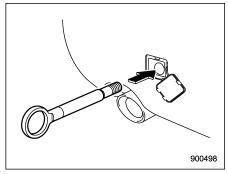
3. Screw the towing hook into the threaded hole until its thread can no
