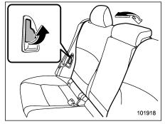
Adjust the seatback to the desired position while pulling the lever.
