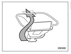
3. Allow the retractor to roll up the belt. You should hold the webbing end and guide it back into the retractor while it is rolling up. Neatly store the tongue plate in the recess and then insert the connector (tongue) plate into the slot.
