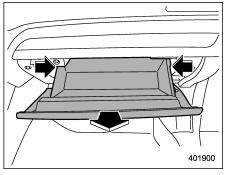
(3) Push both sides of the glove box inward to unlock the stoppers and then pull down the glove box as far as it will go.
