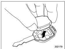
2. Remove the transmitter case from the
