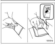
Peel off the anchorage cover from the selected side of the rear seatback to expose the anchorages (bars) to be used for installation of the child restraint system.
