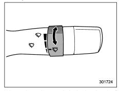
When the wiper switch is in the "position, turn the dial to adjust the operating interval of the wiper. The operating interval can be adjusted in several steps from the shortest interval to the longest.
