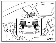
To turn on the map light, press the switch. To turn it off, press the switch again.
