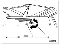
6. Tighten the bolt of the crossbar by using the torque wrench. The tightening
