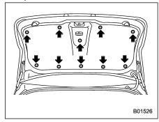
2. Remove the trunk trim lining by removing the clips indicated in the illustration.
