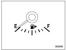
The fuel gauge shows the approximate amount of fuel remaining in the tank. When the ignition switch is in the "LOCK"/
