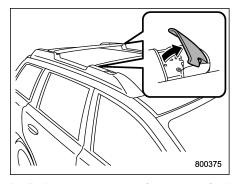
2. Pull out the crossbars from the roof rail holders by pulling up the covers.
