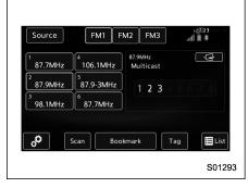
The indication that shows whether the current broadcast is digital or analog is displayed on the top right of the control screen.
