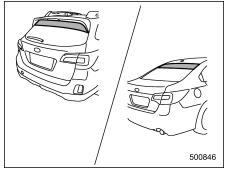
The antenna is printed on the inner surface of the rear window glass.
