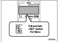
While this screen is selected, pull and hold the "[]/SET" switch to enter the menu screen.
