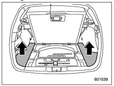
3. Remove the left and right parts of the cargo floor lid.
