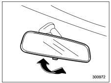
The mirror has a day and night position. Pull the tab at the bottom of the mirror toward you for the night position. Push it away for the day position. The night position reduces glare from headlights.
