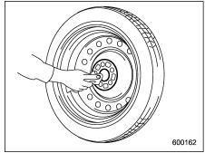
13. Before putting the spare tire on, clean the mounting surface of the wheel and hub with a cloth.
