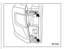
3. Remove the upper and lower screws.
