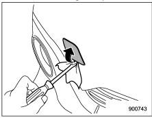
2. Pry off the towing access cover on the front bumper using a screwdriver, and you will find a threaded hole for attaching the towing hook.
