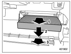
3. Remove the air filter according to the following procedure in order to prevent
