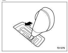
With the vehicle either moving or stationarv. move the select lever from the "D" position to the "M" position to select the manual mode.
