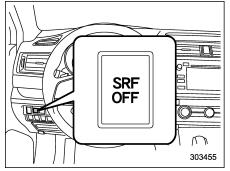
Steering responsive fog lights OFF switch Press this switch to deactivate the steering responsive fog lights system. Press the switch again to activate the system.
