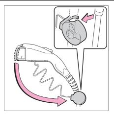
6 Insert the charging connector into the AC charging inlet.
