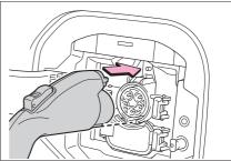
The AC charging connector is locked when the door is locked. If the door is locked and the AC charging connector is plugged in, it will automatically lock.
