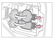
**4** Insert DC charging connector firmly and fully into the charging inlet.
