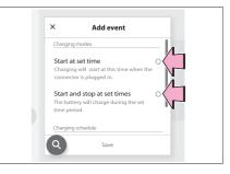
**4** Operate "Start at set time" screen and select desired time, and then select OK .
