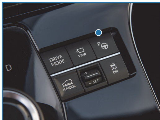
Advanced Park Main Switch
