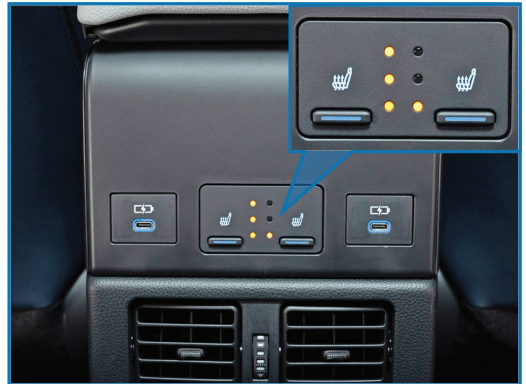
Rear Heated Seat Switches
