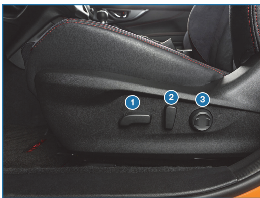
Power Seat Controls
