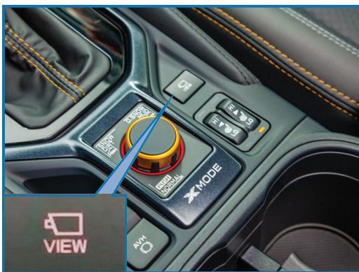
Front View Monitor Switch
