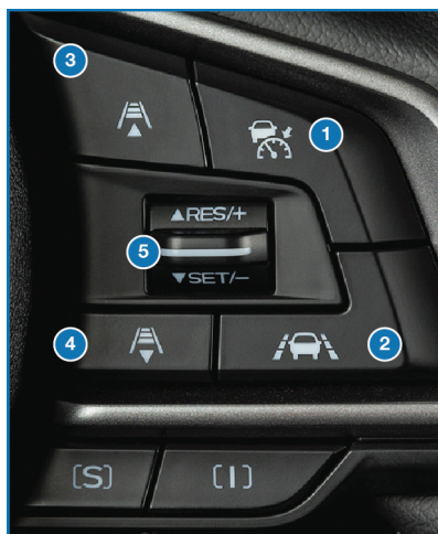
Adaptive Cruise Control Switches
