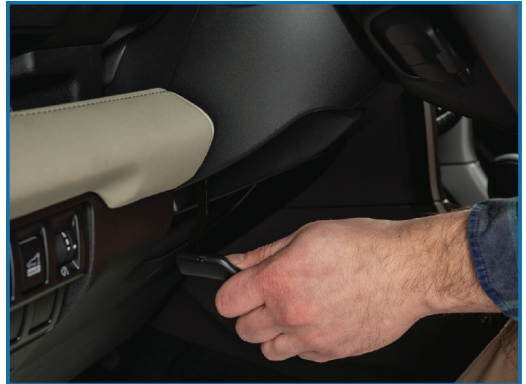
Steering Column Unlock
