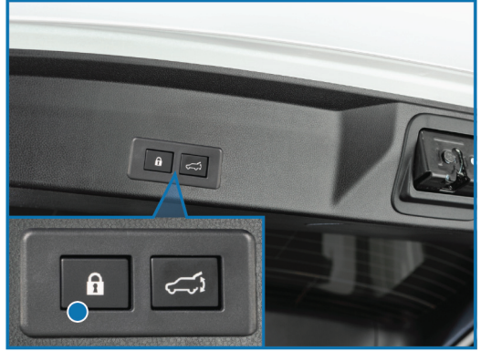
Power Rear Gate Close and Lock Button
