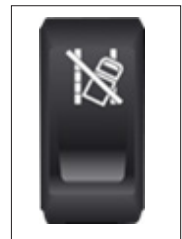
Figure 18 – LDW, HDW, and HDB Disable Switch
