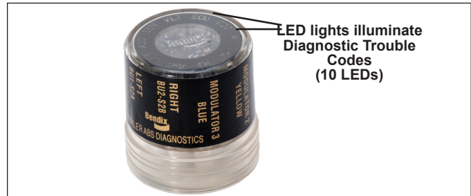
FIGURE 10 - THE BENDIX® TRAILER REMOTE DIAGNOSTIC UNIT (TRDU™)
