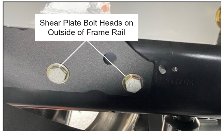
Figure 3 — Shear Plate Bolts with Heads Outside
