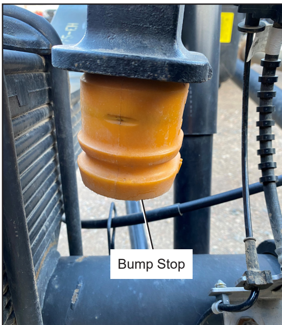
Figure 16 — Ford Rear Suspension Bump Stop
