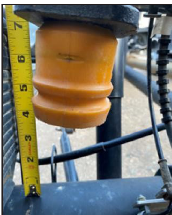
Figure 17 — Ford or Dodge Measuring for Suspension Travel Number
