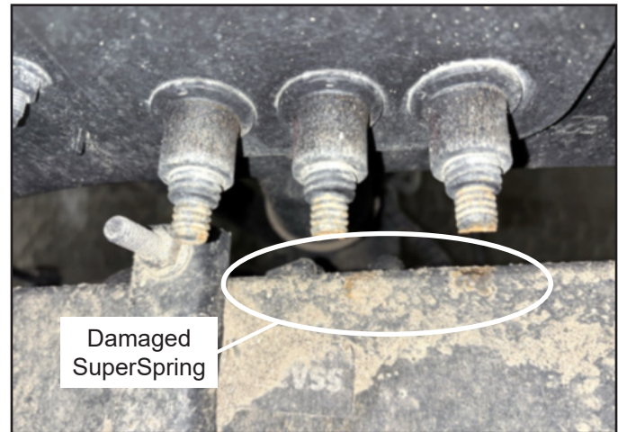
Figure 10 — Indents on Leaf from Bolt Contact
