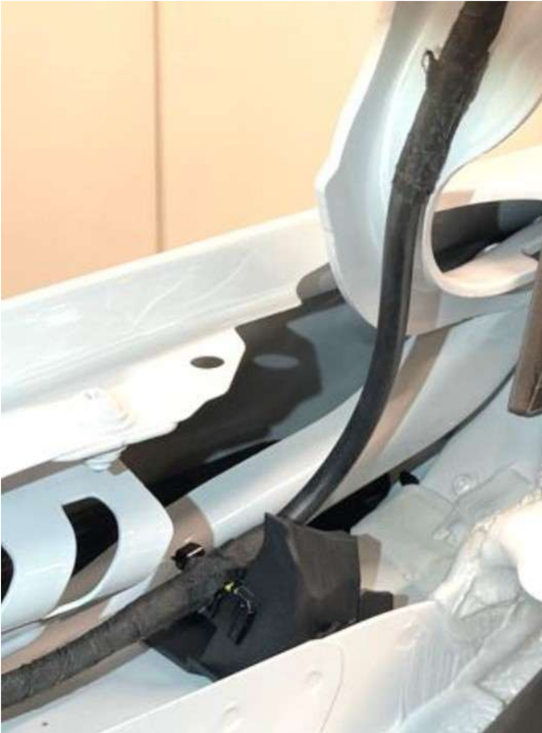
Figure 2. Correct routing of washer fluid hose.
