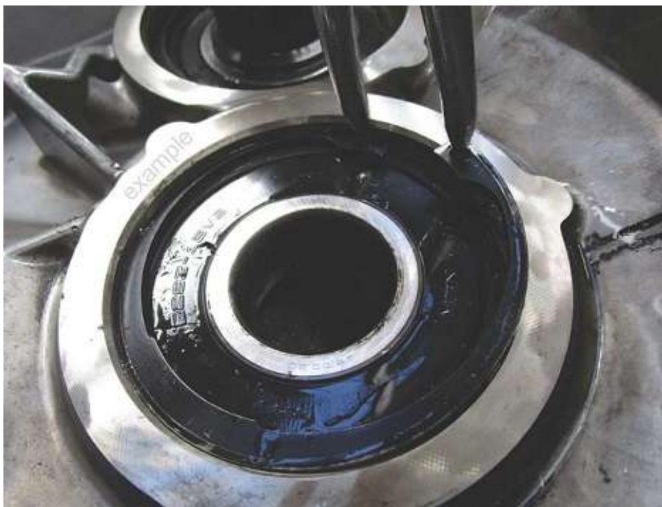
Figure 9. Removing the retaining ring (example).
