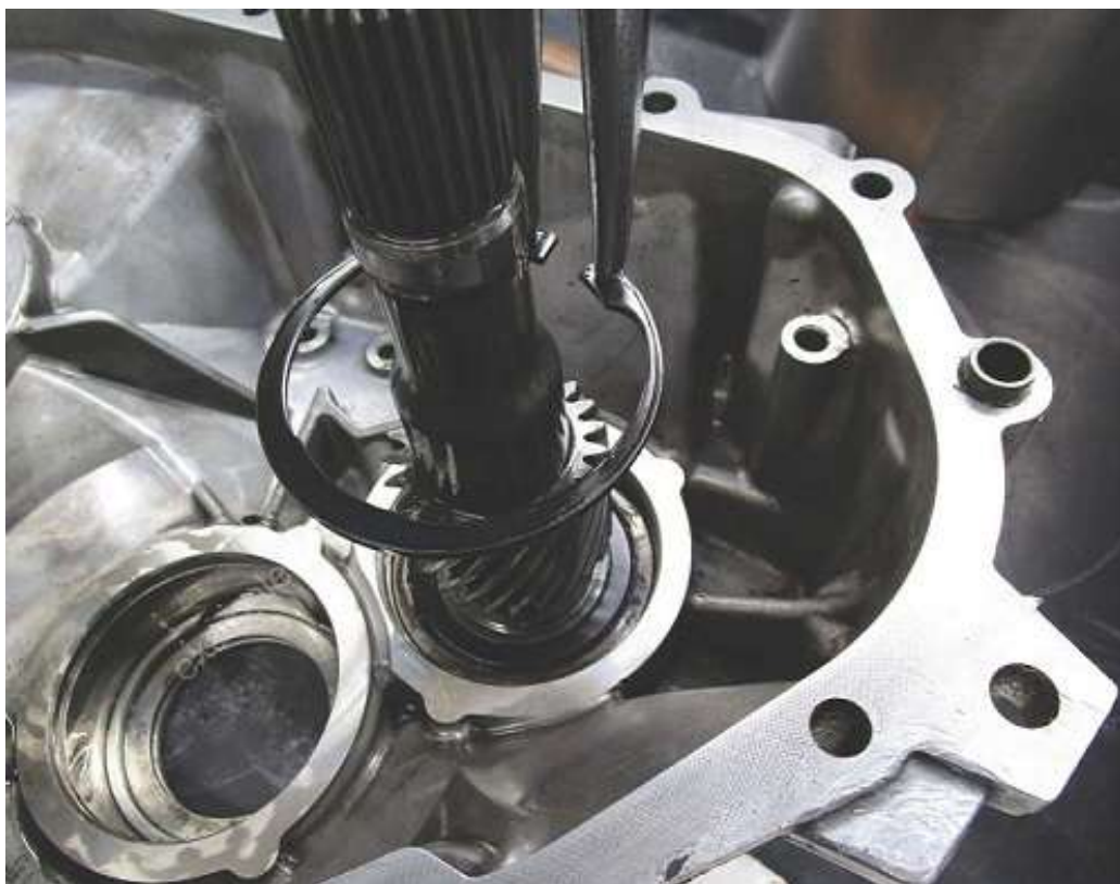
Figure 11. Removing the outer retaining ring for the drive shaft (example).
