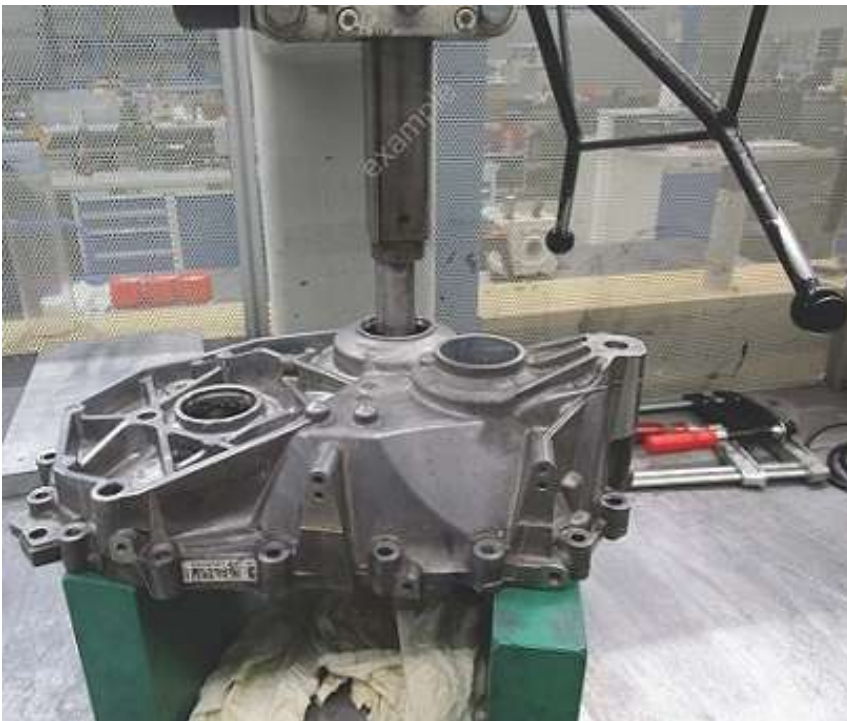
Figure 8. Pressing out the intermediate shaft (example).
