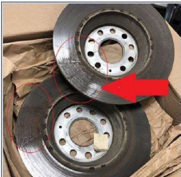
Figure 7: Corrosion, brake pad stuck to brake rotor.
