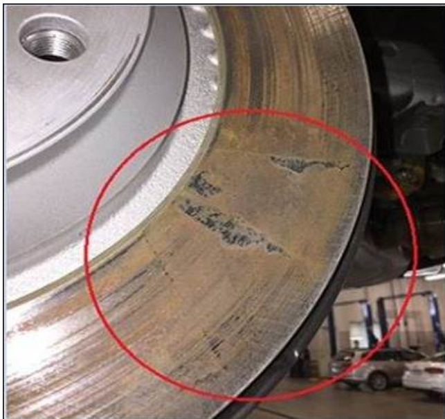
Figure 7: Corrosion, brake pad stuck to brake rotor.
