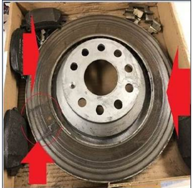
Figure 6: Corrosion, brake pad stuck to brake rotor.
