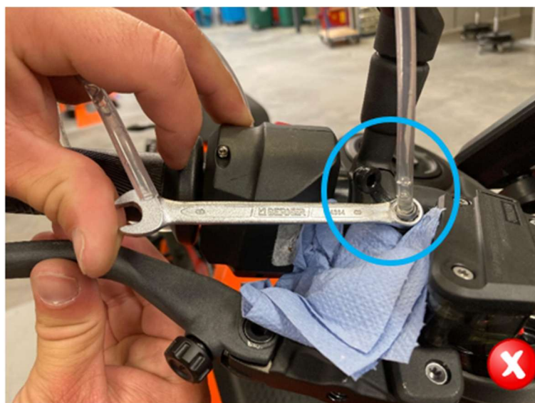
Fig.2 – Air in the master cylinder of the front brake system
