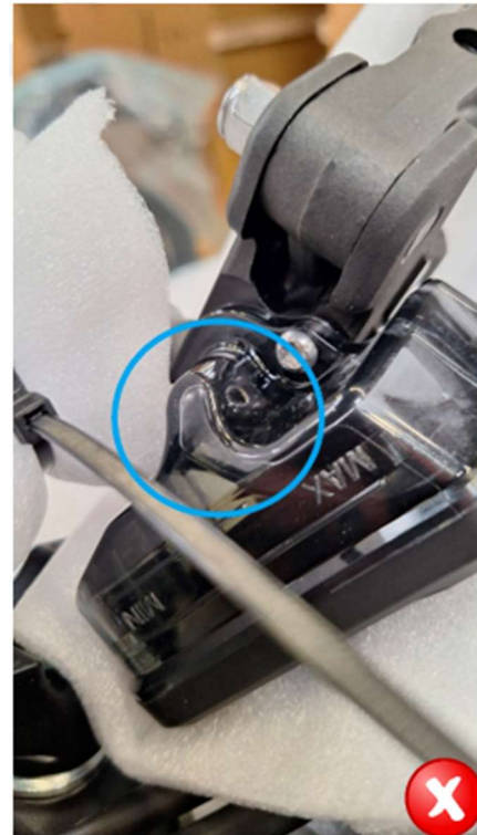
Fig.1 – Incorrectly packaged KTM 390 DUKE MY2026. Air can enter the master cylinder of the front brake system.
