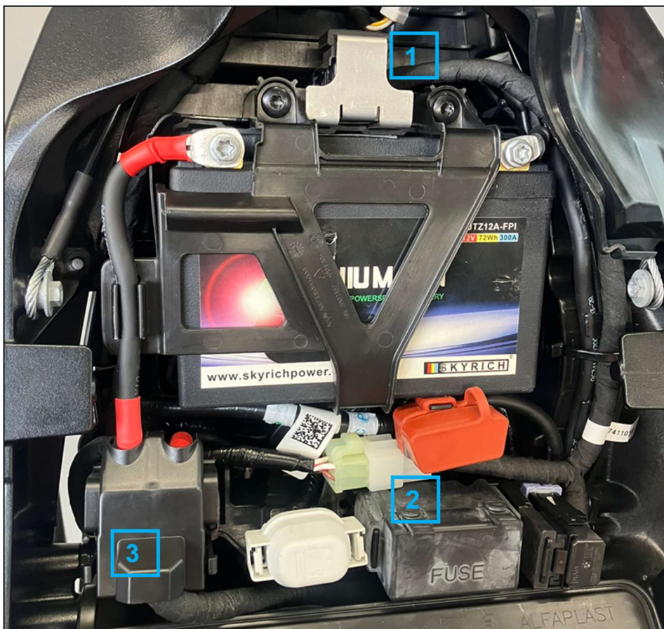
Fig. 8 – Mounted adapter cable start relay
