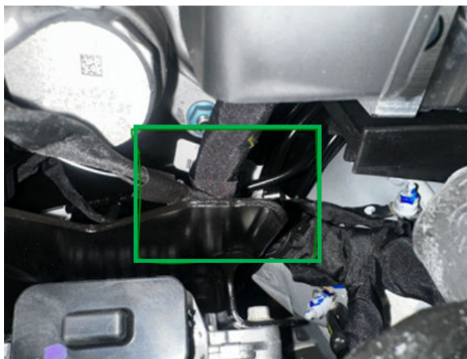
Fig. 2 Correctly Routed Harness
