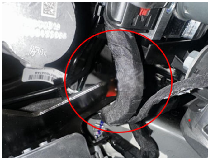
Fig. 1 Incorrectly Routed Harness
