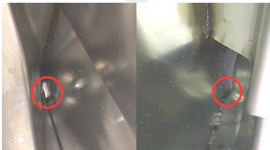
Figure 17 – Do not block the drain holes at the front and rear ends of the door panel
