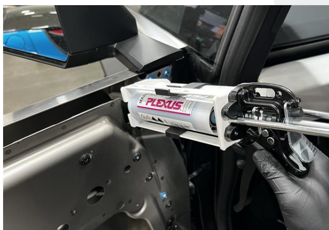
Figure 15 – Apply adhesive to front door side mirror bracket
