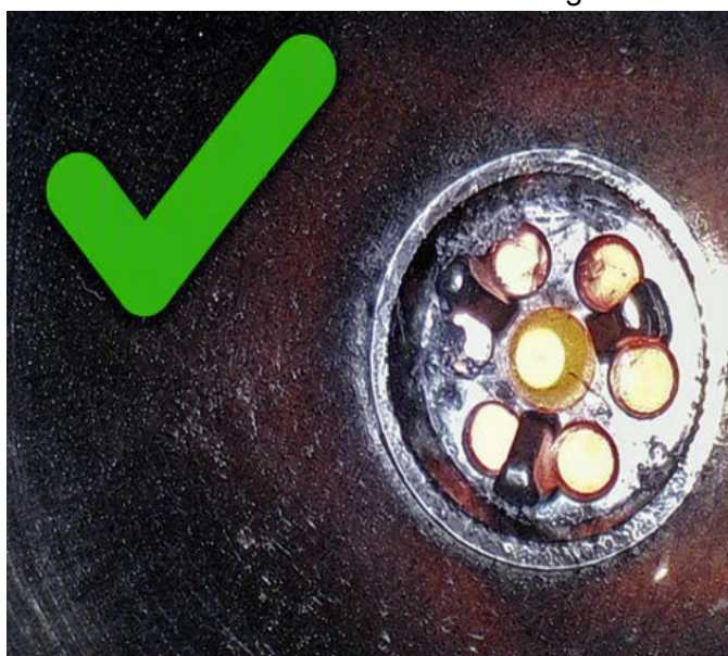
Fig. 6 Umbrella Valve Seal - Present
