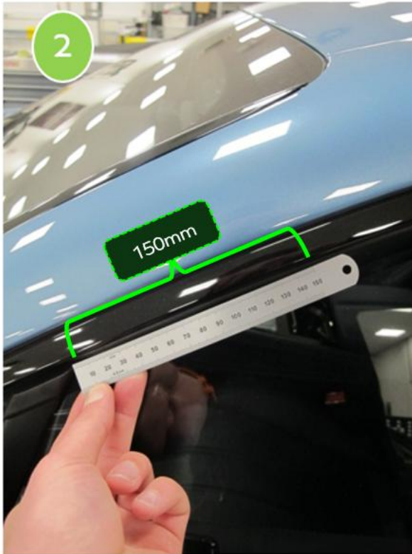
150mm behind front div bar
