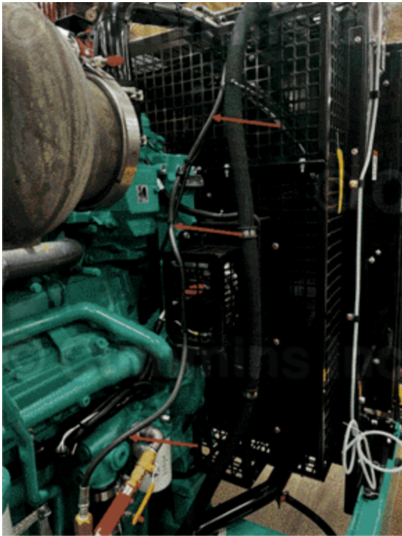
Figure 2, Cracking Location on Heater Vent Hose
