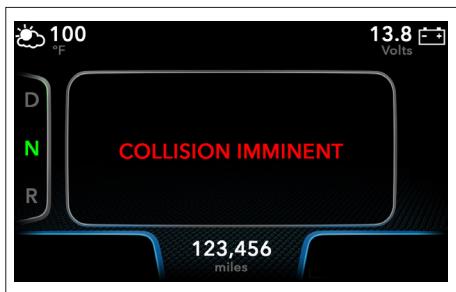
Figure 16 – AEB System Alert and Possible AEB Applied
