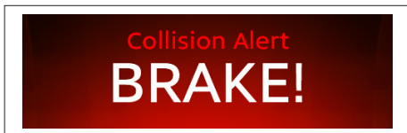
Figure 15a – AEB System Alert
