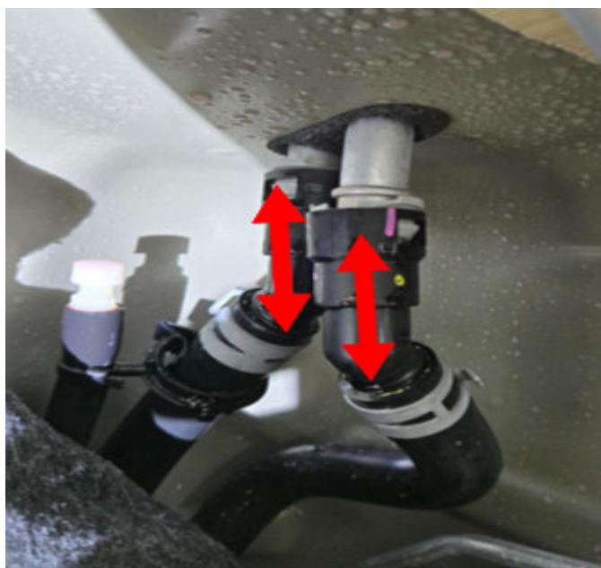
Fig. 3 Rear Coolant Hose Inspection
