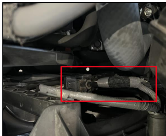
Figure 2. Close-up of the Cooling Fan Plug
