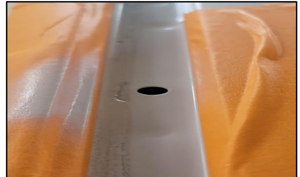
Figure 3. Clip Hole After Sanding and Painting.
