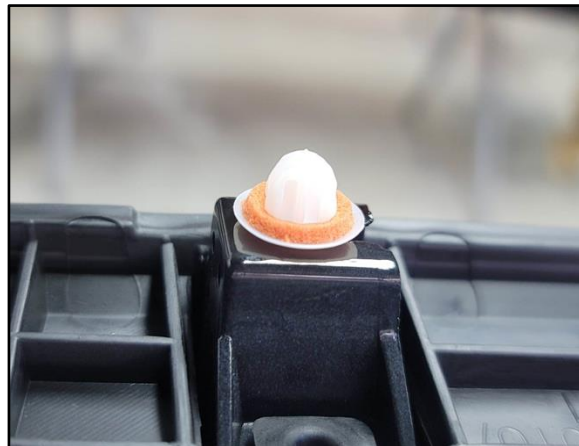
Figure 4. New Roof Rail Garnish Clip
