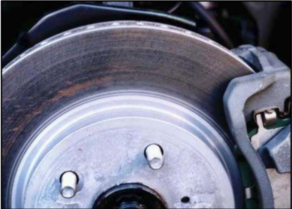
Figure 2. Slight Rust on Rotor (Easy to Remove by Braking)
