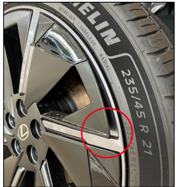
Figure 9. Incorrectly Installed Wheel Cap
