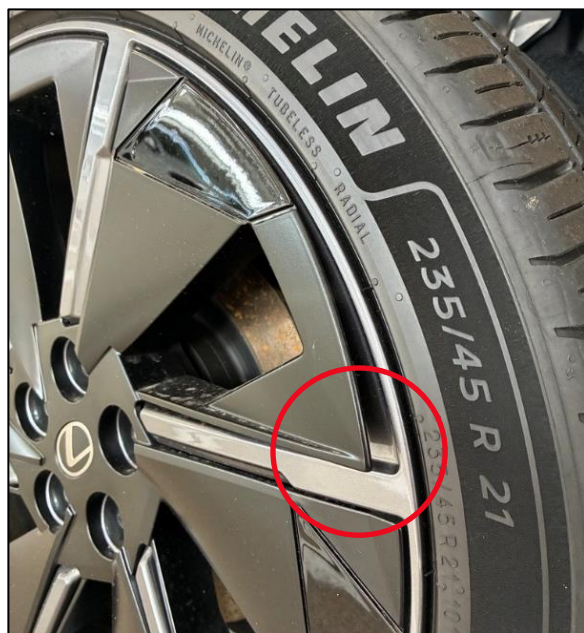
Figure 9. Incorrectly Installed Wheel Cap
