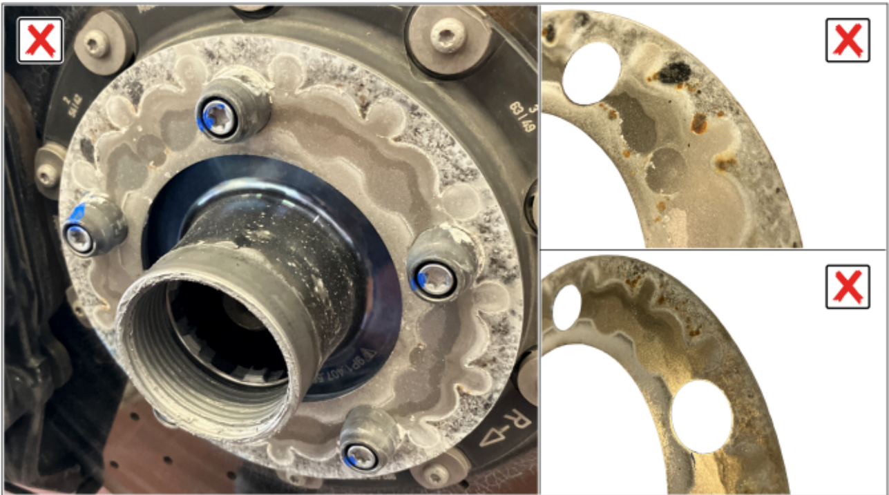
Limit sample illustrations for abrasion and corrosion of the friction plate
