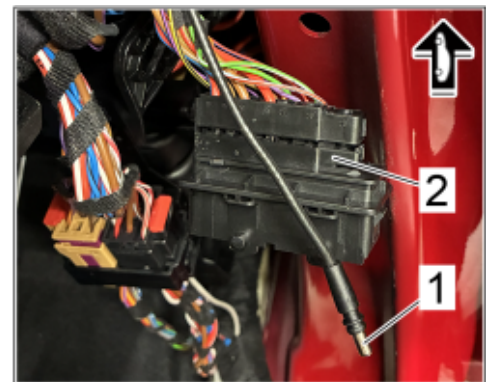
Signal line for door connection point
