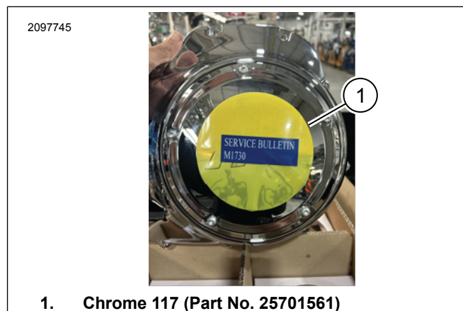
Figure 1. Incorrect Derby Cover
