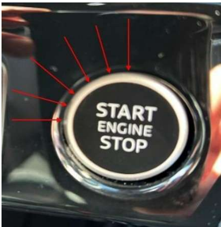
Figure 1. The start/stop button is not aligned correctly.
