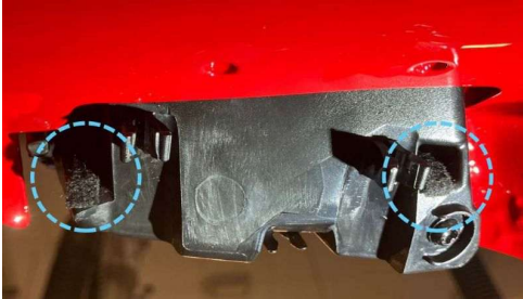
Figure 2. Felt strips applied to locking pins.
