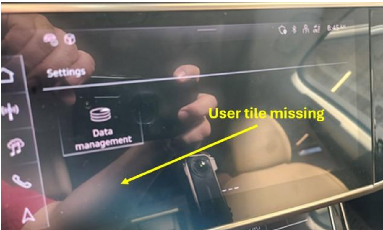
Figure 2. The user tile is missing.
