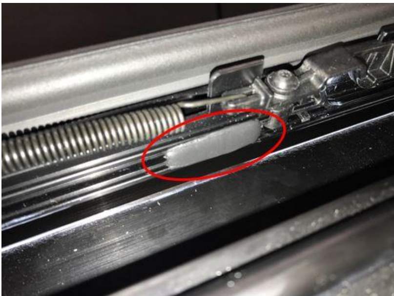
Figure 32. Apply the butyl barrier into the guide rail channel.
