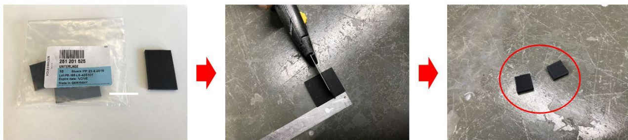
Figure 25. Cut the rubber buffer to size.
