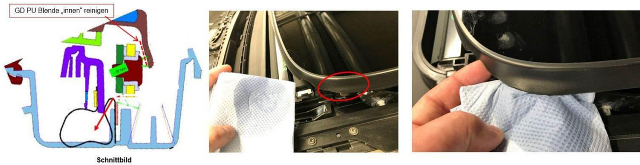
Figure 23. Clean the inside of the glass panel with cleaning solution.
