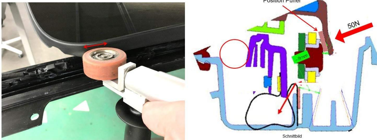
Figure 27. Press down on the rubber buffers.
