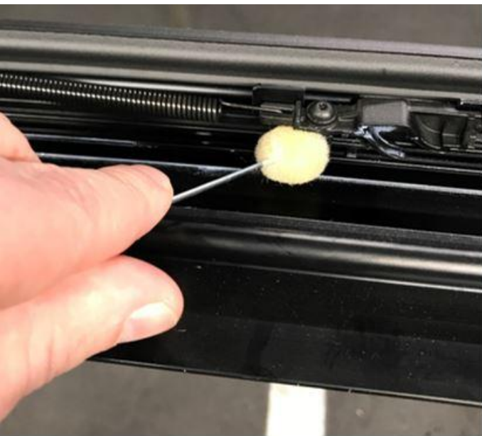
Figure 29. Clean the area with a cleaning solution.
