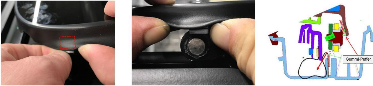
Figure 26. Attach the rubber buffers to the trim.
