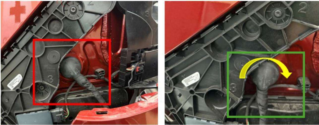
Figure 4. Left – factory grommet orientation. Right - bumper wiring harness grommet in 6 o'clock position.
