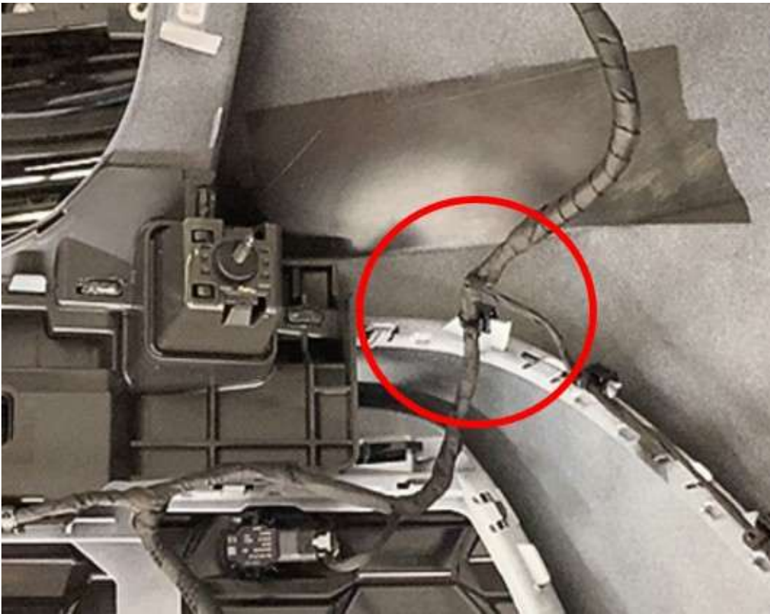
Figure 2. Position of cable tie with clamping base
