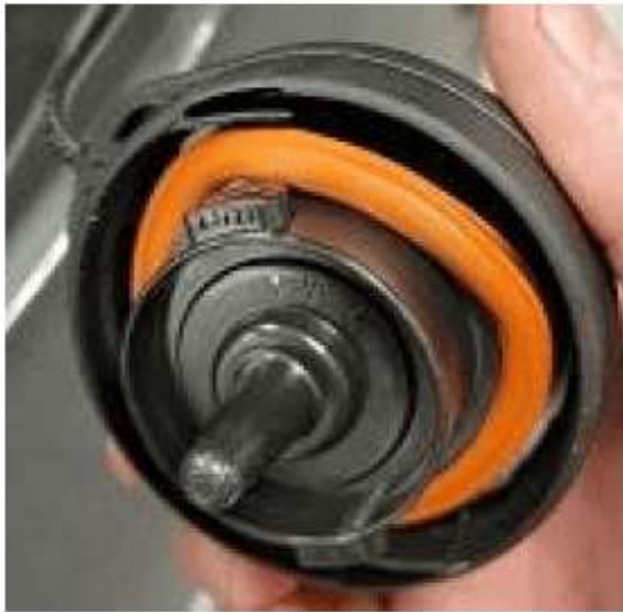
Figure 1. The seal (orange) is twisted.
