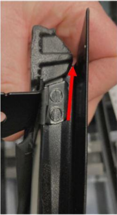
Figure 2. Gap between foam piece and the guide.
