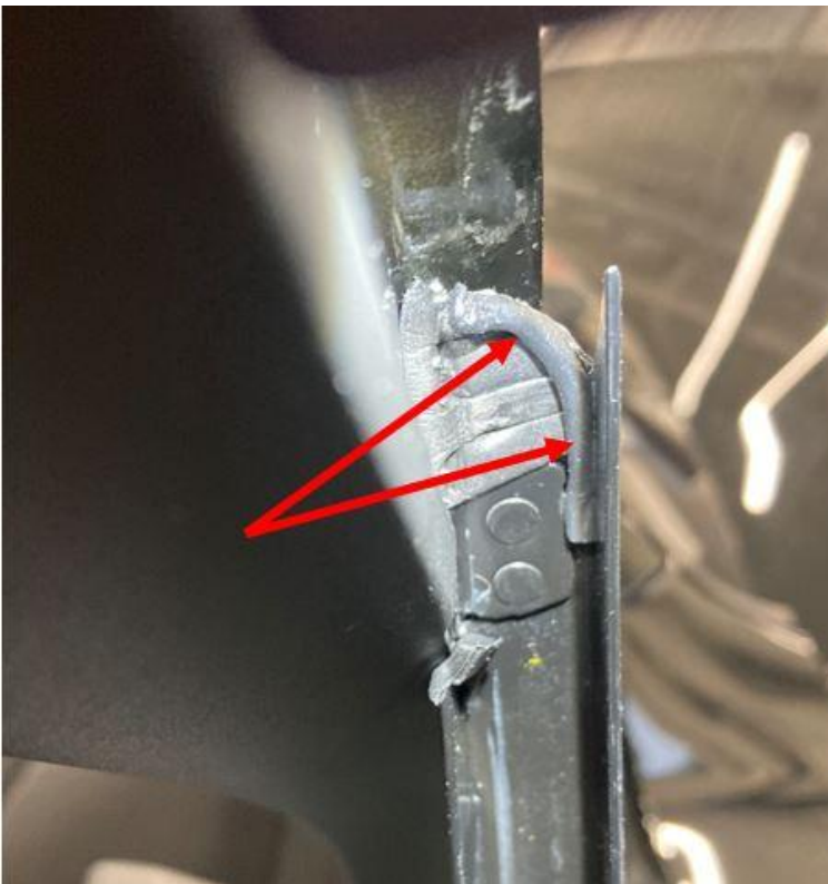
Figure 3. Press the butyl cord into the transition area between the foam piece and the door.
