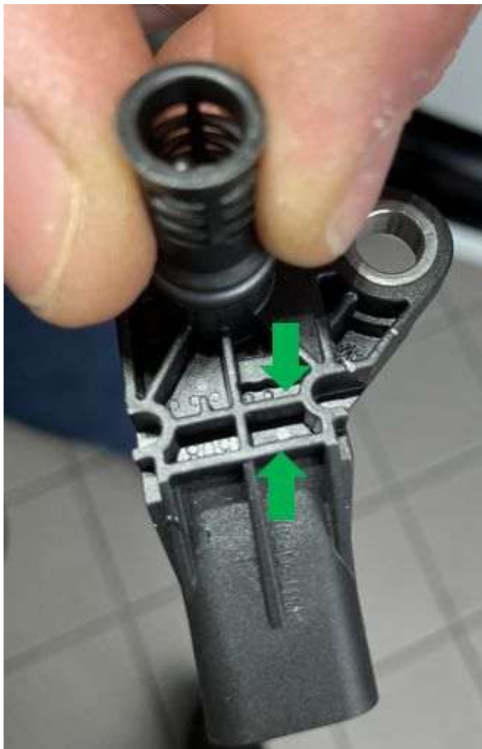
Figure 1. Apply the adhesive bead as indicated by the green arrows.
