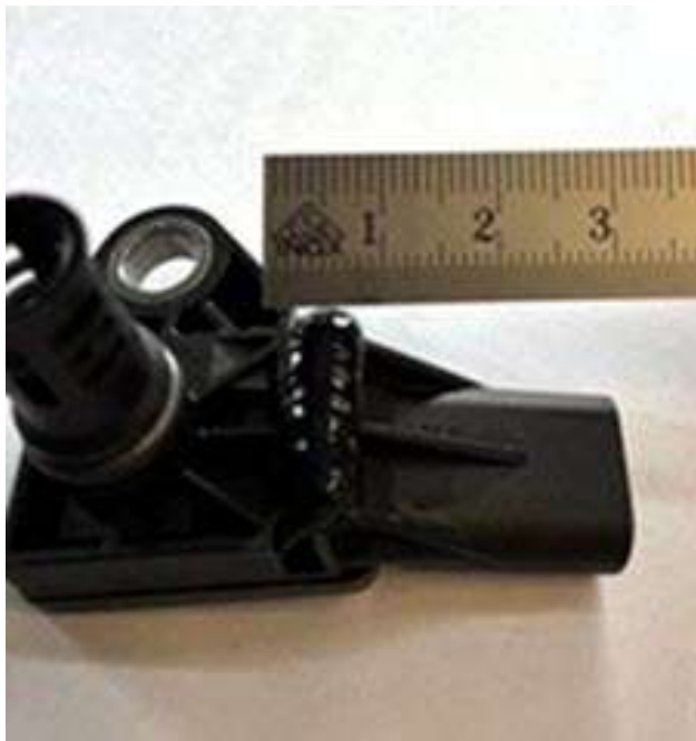
Figure 2. The adhesive bead should be approximately 5mm wide.
