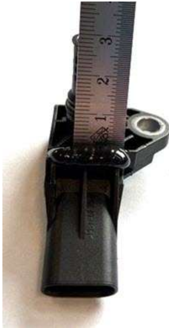
Figure 3. The adhesive bead should be approximately 2 mm high.
