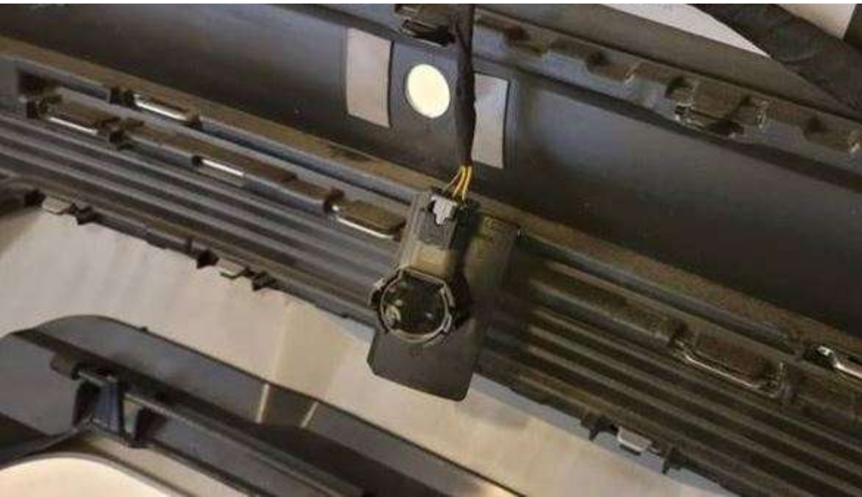
Figure 2. Retaining plate for parking sensor hanging loose.
