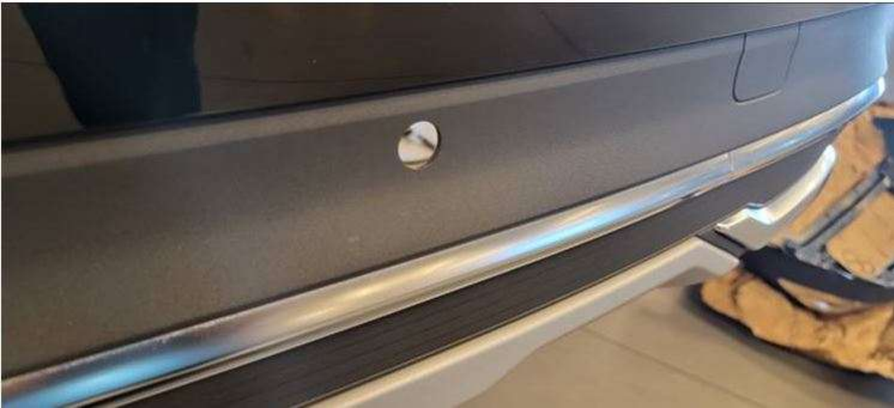
Figure 1. Retaining plate for parking sensor has come loose.
