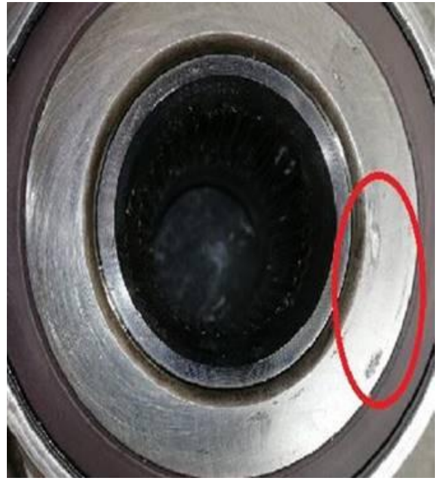
Figure 5: Metallic particles/damage in the wheel hub/bearing.
