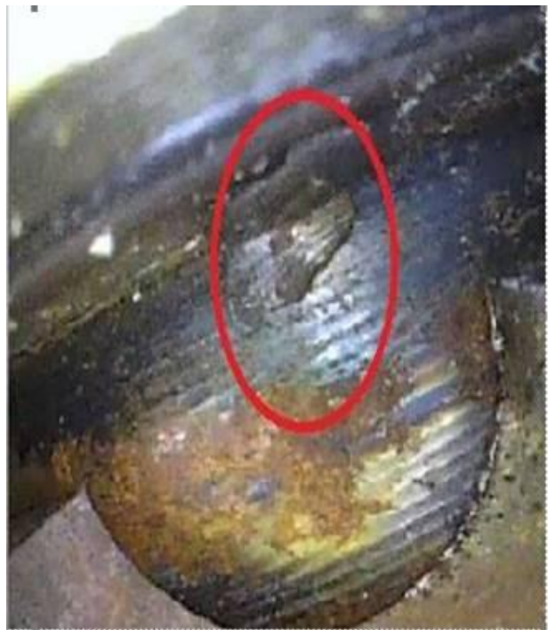
Figure 3: Metallic particles in the hub.
