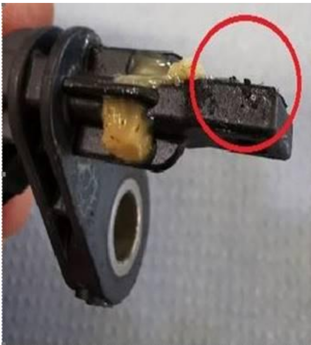
Figure 2: Metallic particles in the speed sensor.
