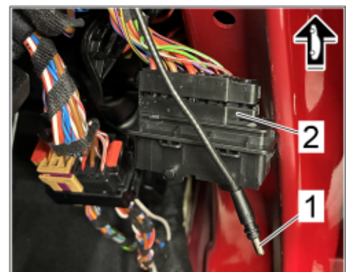
Signal line for door connection point
