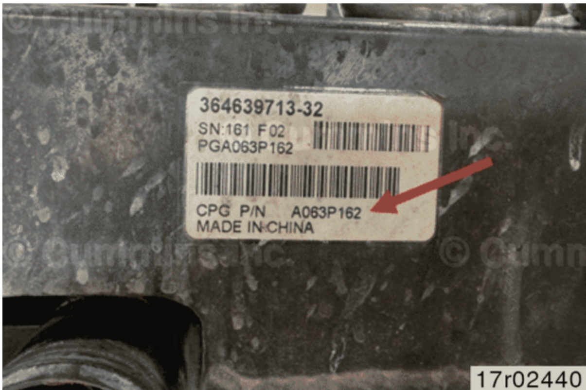
Figure 2, A063P162 Part Number Location, Not Covered in the TRP
