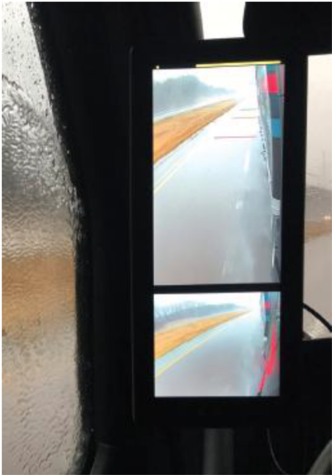
Inclement Weather Visibility (road spray and window soiling)
