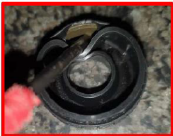
Damaged outer lip, delamination between rubber and metal skeleton
